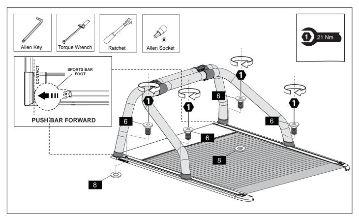
4. Push the sports bar forward so that the front feet are aligned with the front of the corner cap as shown. Reposition the M8 T Nuts (7) in the T-channel to align with the holes in the Foot Plates (1),(2),(3),(4). Place a washer (8) under front foot and then secure the sportsbar in place with four M8 Counter Sunk Socked Head Screws (6). Torque to 21Nm.
