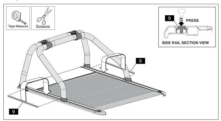
5. Measure the distance between the feet in the side rail channels and cut the T-Channel Extrusion (9) to length. Fit the T-Channel Extrusion into the side rail channels between the Sports Bar legs, by firmly pressing it into the channel recess.
