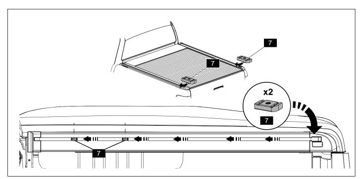
**3.** Slide two M8 T Nuts (7) into the RHS and two into the LHS T-channel of the side rails as shown. Ensure they align roughly with the holes in the Front and Rear Side Plate on the feet of the sports bar.
