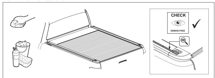
1. Prepare the surface of the side rails by cleaning them thoroughly ensuring that any debris in the side rail channels is completely removed.
