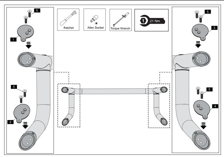
2. Attach the adaptor kit brackets (1),(2),(3),(4) to the respective feet as shown with the M8x25 Counter Sunk Socked Head Screws (5). Torque all screws to 21Nm.
