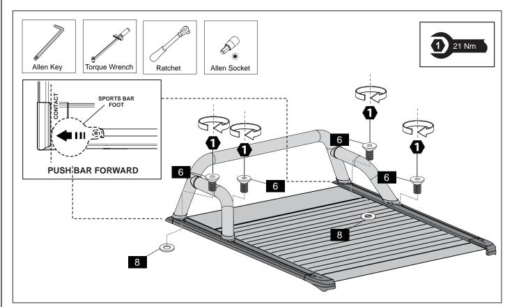
4. Push the sports bar forward so that the front feet are aligned with the front of the corner cap as shown.
