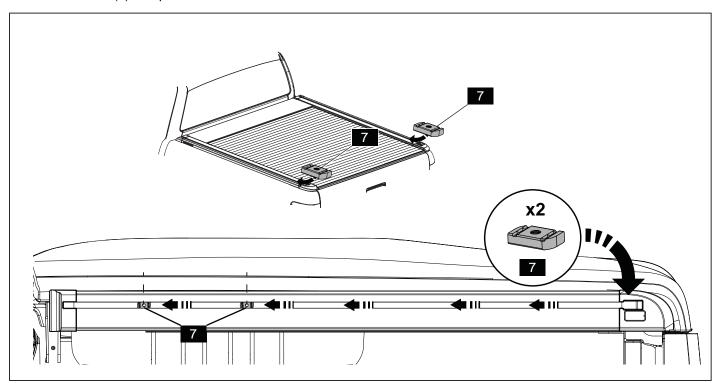
**3.** Slide two M8 T Nuts (7) into the RHS and two into the LHS T-channel of the side rails as shown. Ensure they align roughly with the holes in the Front and Rear Side Plate on the feet of the sports bar.
